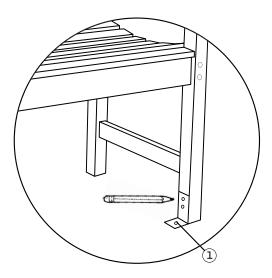
**STEP 2**Drill concrete pad. Drill legs.
